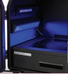
Blue light - LED epiillumination module allows visualisation of some stains with better clarity and without DNA damage – e.g. runSAFE
