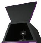
Autoradiographs – high resolution 5MP camera captures images in high detail, especially when scrutinising separation between closely located bands or spots
