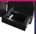
DNA - use the slide-out UV transilluminator to capture images of DNA gels stained with EtBr and SYBR dyes
