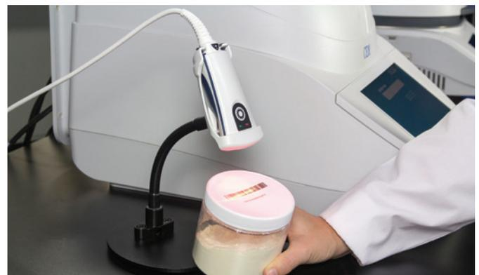
A barcode scanner is included with each system. This enables you to automatically import customer codes into sample ID's.
